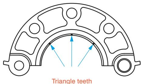
2. Flange adapters 7041 have small triangular teeth inside the wedge arm to prevent the pipe from rotating. The teeth should be ground in the event of a connection with a flange with a rubber coating.
