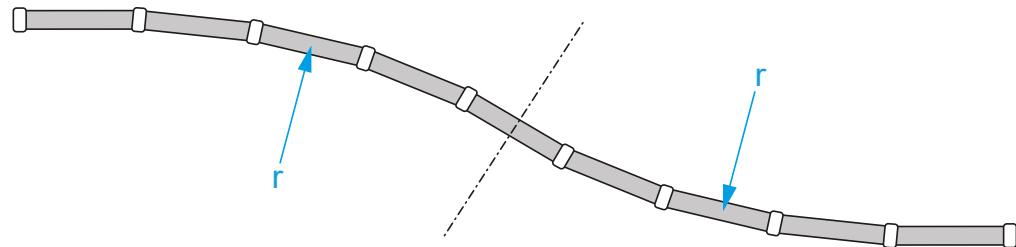
For example, using a 100 mm (4") 7705 coupling in the pipeline shown in the diagram, the maximum permissible deflection ( $\theta$ ) of the coupling will be 3.4°, the pipe length (l) will be 5.5 meters and the radius of curvature (R) reaches 92.7 meters.
