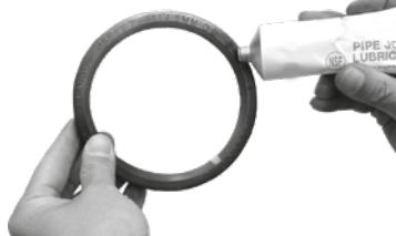
**Check the gasket grade and lubricate it:** Check the colour of the gasket strip and make sure that the gasket supplied is suitable for the intended use. Then apply a thin layer of grease to the lip of the gasket.
