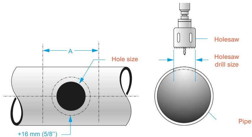
When installing saddle and cross type couplings, it is required to prepare the pipe by making the hole. This method of pipe preparation requires cutting or drilling a certain hole dimension in the pipe axis. Always use the right dimension keyhole saw as shown in this document.
