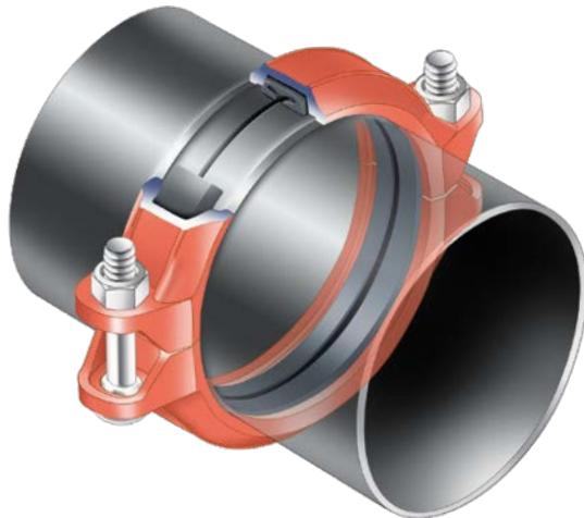
**Flexible couplings** are designed to adapt to axial movements, rotational movement and angular movement of a minimum of one degree. Flexible couplings are used in applications where pipework is a curved and deformed structure or in which pipeline systems are exposed to external forces beyond normal static conditions, such as seismic events or when there is a problem of excessive exposure to vibrations or noise.
