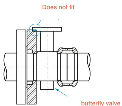
4. When installing the flange adapter 7041 on the butterfly valve or ball valve, make sure that the outer diameter of the flange adapters does not interfere with the valve actuator or the actuator mounting washer.
