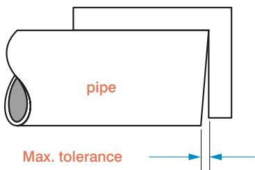
Maximum permissible tolerances for ends cut at right angle:
