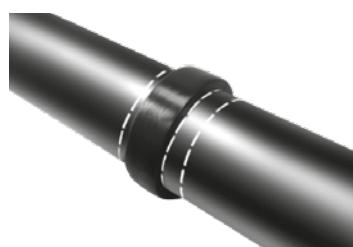
**Install the gasket:** Place the gasket on the ends of the pipes and centre it between the first marks marked on the inside. The ends of the pipes should always come into contact.
