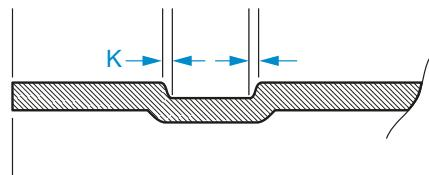
Grooves made by rolling should be defined as clearly as possible. To obtain the optimal coupling performance, "K" dimension should be as small as possible. During the grooving process, the machine operator should set the feed force of the upper roll set to obtain the best possible groove profile.
