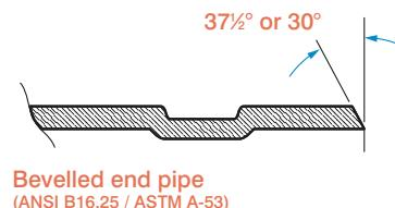
Although pipes with plain-ends are preferred, the use of a bevelled pipe is permissible provided that the wall thickness is 9.5 mm or less and the bevel is  $37\frac{1}{2} \pm 2\frac{1}{2}$ ° or 30°, according to ANSI B16.25 and ASTM A-53.
