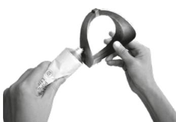
**Check the gasket grade and lubricate it:** Check the colour of the gasket strip and make sure that the gasket supplied is suitable for the intended use. Then apply a thin layer of grease to the lip of the gasket. The standard, factory-supplied gasket is made of a mix of E-type EPDM. It is marked with a green strip and is generally suitable for use in water pipelines.
