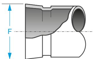
The diameter of the pipe end, which may expand during rolling, should be within the specified tolerance at the extreme end of the pipe.
