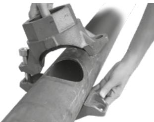
**Position the upper casing in the correct position:** Place the upper casing part on the pipe so that the retaining flange fits properly into the hole. Then add the lower casing part from the opposite side of the pipe.
