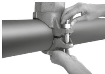
**Insert the bolts and put on the nuts:** Insert the remaining bolt and tighten the nut manually. Make sure that the oval bolt head is locked in the bolt hole in the coupling casing.
