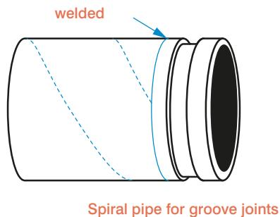
Spirally welded pipes are acceptable as long as the welding beads have been removed from the gasket placement surface. It is also permissible and recommended to weld a grooved part with the coupling to the pipe end. Each time after removing welding beads from the surface of the gasket seat, care should be taken to avoid excessive grinding of the surface. After grinding the surface should always be covered with anti-corrosion coating.
