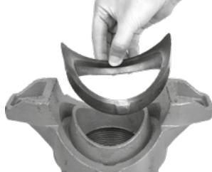
**Insert the gasket:** Insert the gasket into the gasket seat in the casing. The retaining projections on both sides of the gasket should properly fit into the recesses.
