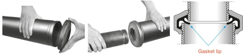
**First, install the gasket on the larger pipe:** Place a larger gasket opening on the larger end of the pipe and match both pipes to be joined. Insert the smaller pipe into the gasket. The gentle torsional movement will help to match the gasket to the pipe. The gasket should not protrude beyond the end of the pipe or its groove.
