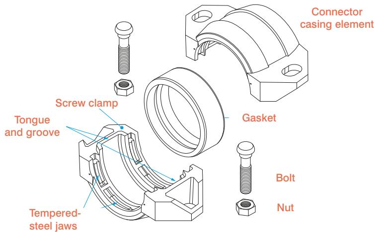
The KAN-therm Groove coupling with a smooth end of Wildcat type (model 79) has been designed for mechanical joining of carbon steel pipes with smooth ends or bevelled. Grooving is not required. The Wildcat coupling (model 79) is recommended for use on carbon steel pipes with hardness less than HB150. It is not recommended for use on stainless steel, plastic, HDPE, cast iron and other brittle materials.
