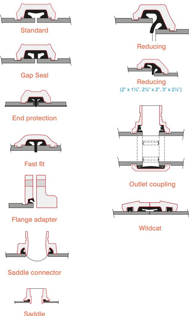
Proper selection of gaskets is essential for optimum performance of grooved couplings, flange adapters and saddle connectors. KAN-therm Groove couplings are used with various types of gaskets: standard, GapSeal (slotted), EP (with end-protection) and FF (quick-release). GapSeal gaskets are compatible with standard gaskets and can be used interchangeably. Always use gaskets that match the selected coupling model.
